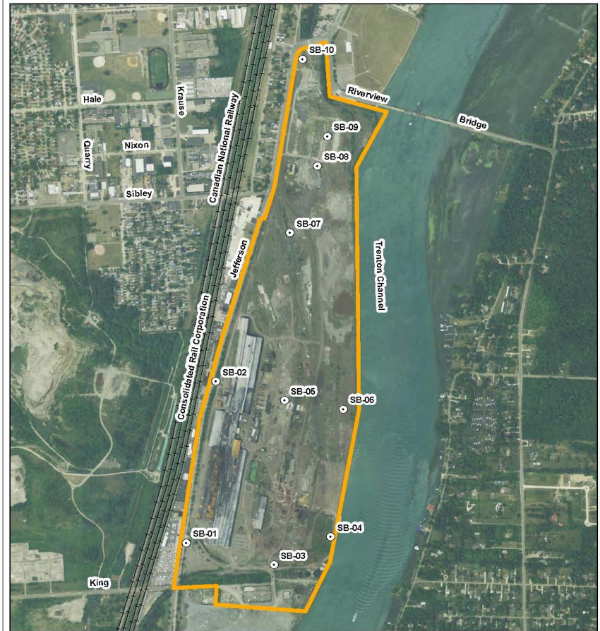
FIGURE 5 SOIL BORING SAMPLING LOCATIONS
