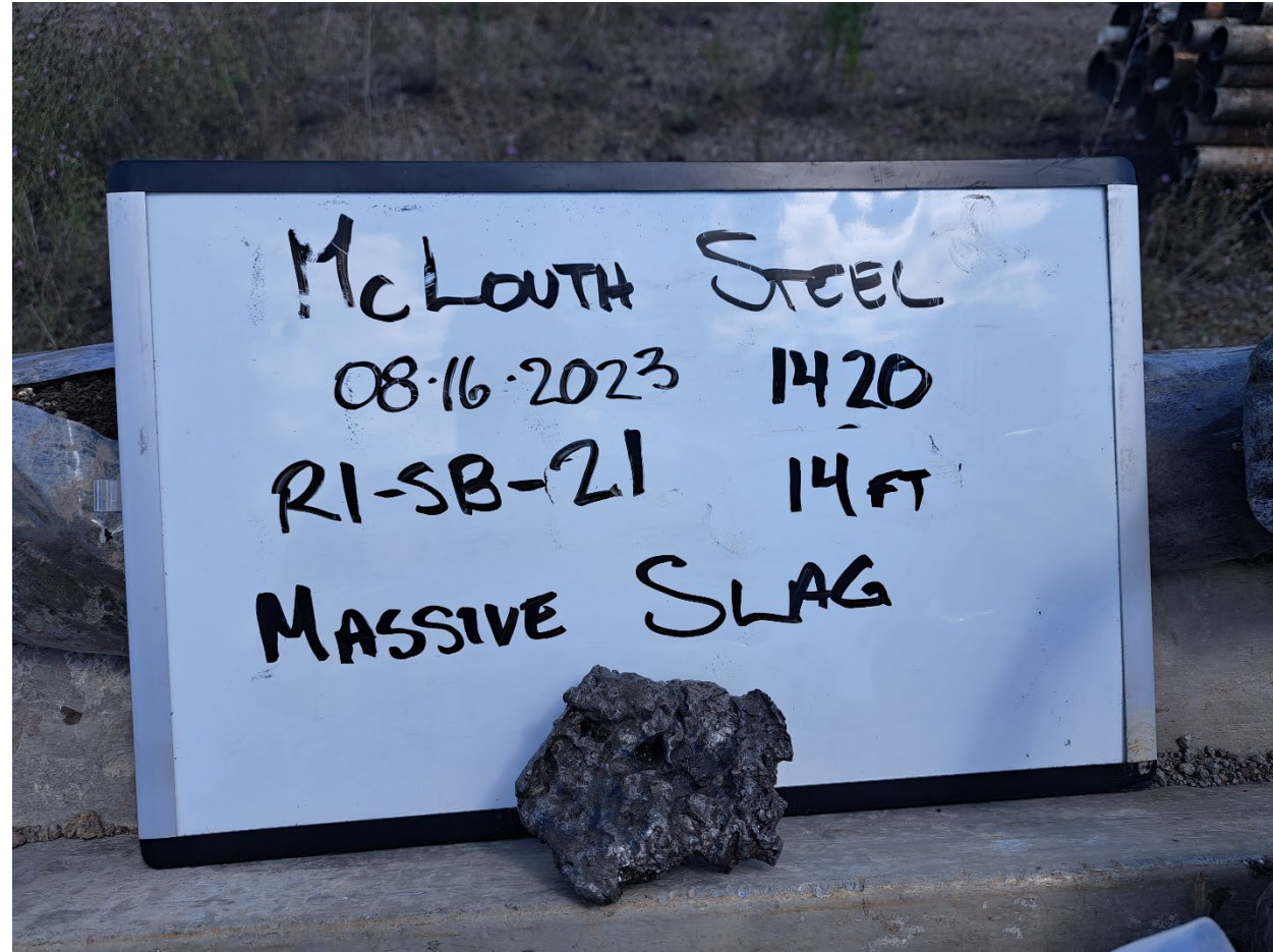
Images of a soil boring soil sample being screened for volatile organic compounds and an example of steel plant slag
